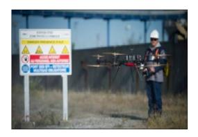
It took 18 months collaboration with French Ex design consultancy CentrExpert to upgrade one of the company's existing drones and make it ATEX compliant. Changes included replacing carbonfibre propellers with wooden ones to reduce static risk, adapting all electrical and electronic systems and making modifications to the wiring.
