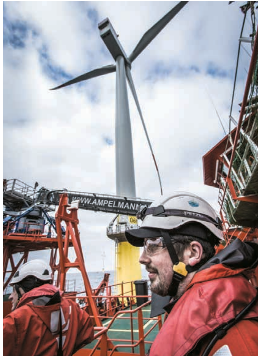
The Ampelmann system also offers the perfect addition to the special seaworthiness of the SOVs: It compensates for wave motion, making access to the wind turbines possible even during storms. With standard vessels, access was only possible up to swells of 1.5 meters.
