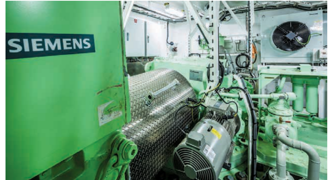
The Diesel-electric engine of the vessel propels the SOV Faraday at up to 14 knots (around 26 kilometers per hour) into the open sea. The electric power is supplied by Siemens Generators.
