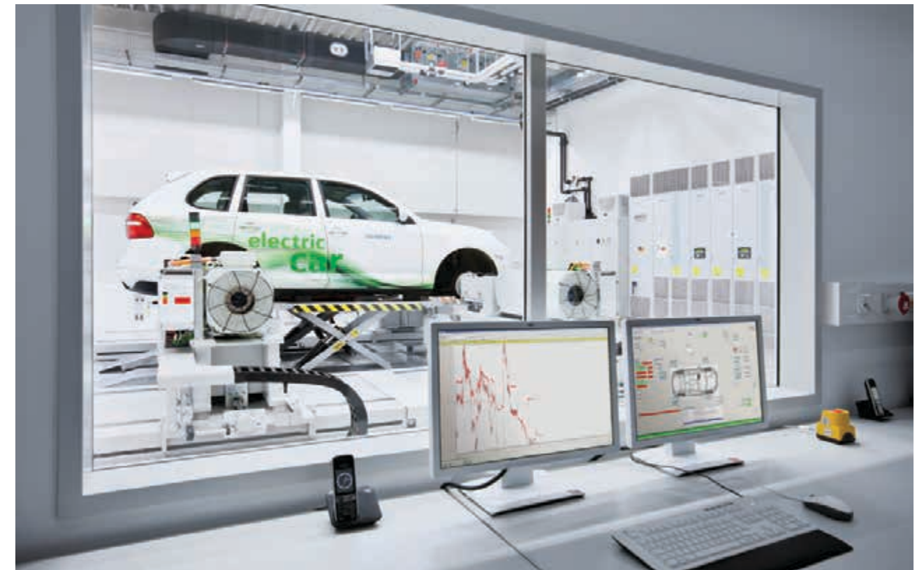
The Siemens test rig at the new eCar Powertrain Systems Business Unit production and development site in Erlangen enables the handling performance of electric vehicles to be simulated in a range of different situations. This is where Siemens tests the components for its SIVETEC electric integrated drive units.
