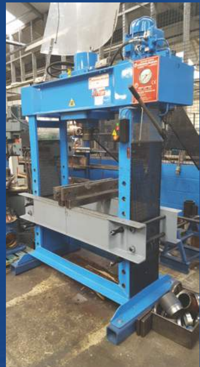
A new investment for the company, a 120 ton vertical press.
