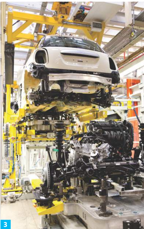
1. Robots welding the side frame for the new 5-door MINI in Plant Oxford's bodyshop. 2. Ian Baxter and Steve Leng of Morgan Advanced Materials with Alex Page of Mid Kent Electrical. 3. At engine marriage as the engine is lifted up under the car for fitment.
