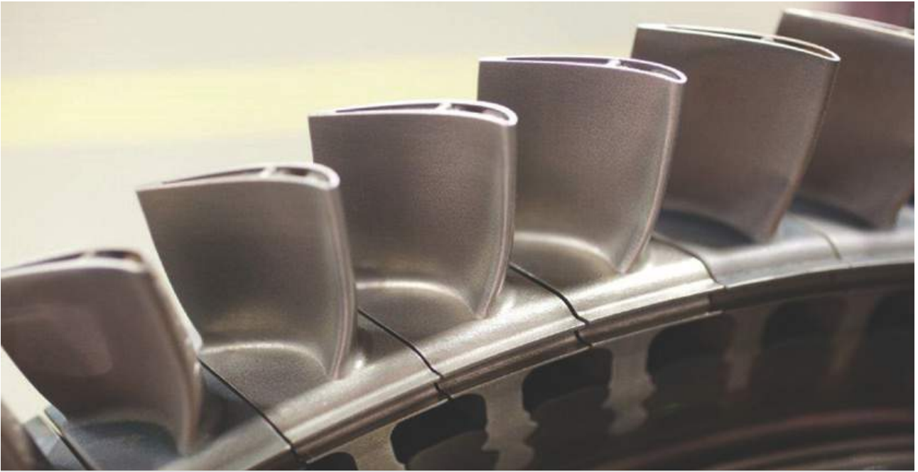
The blades had to endure 13,000 revolutions per minute and temperatures beyond 1,250 degrees Celsius.
