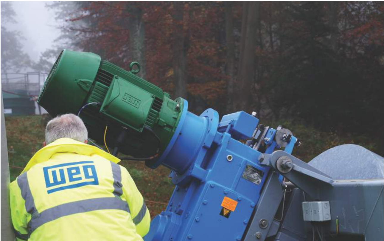
The lighting for the entire house can now be powered using the high efficiency WEG IE3 electric motor driven over-speed as a generator.
