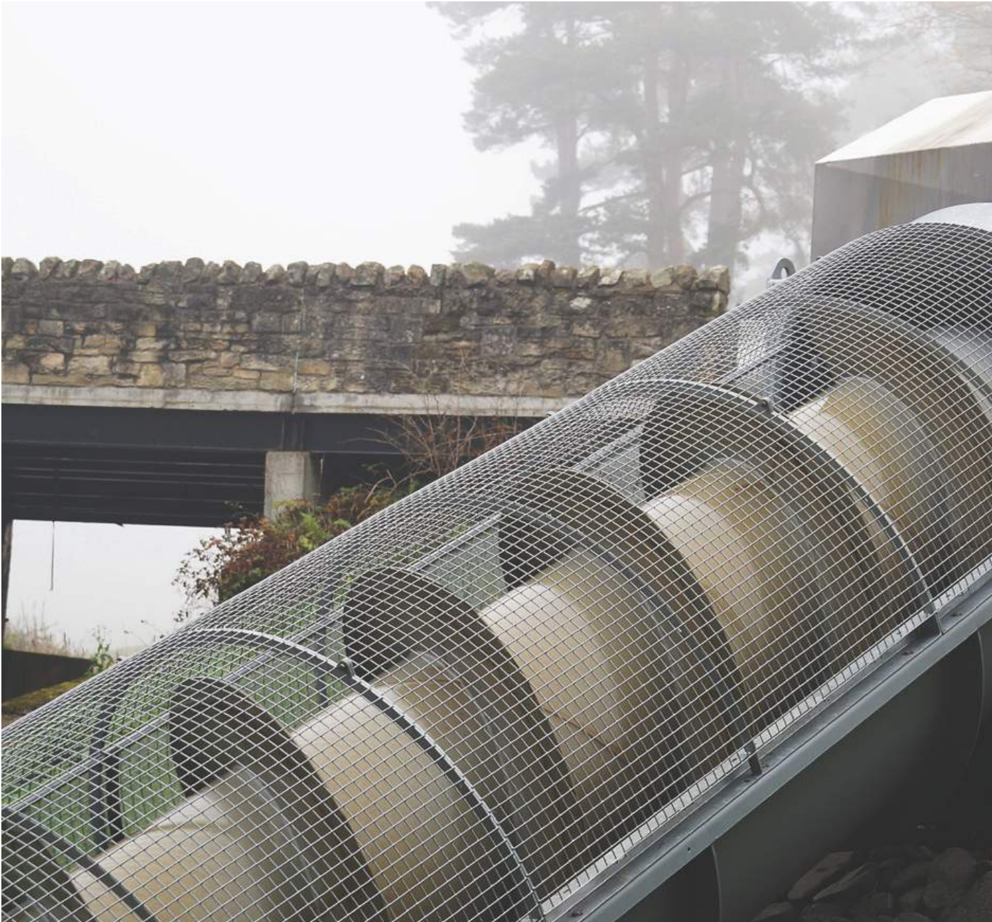
An Archimedes screw, although ancient in principle, is actually a very efficient way of generating power when you have a large volume or flow of water, but low head.
