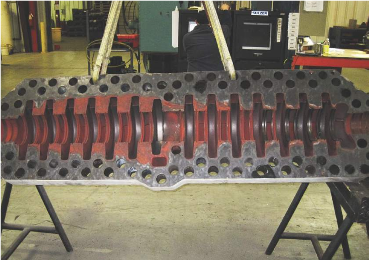
When a pump operates in a boiler feed system, iron oxide deposits are often found in the casing
