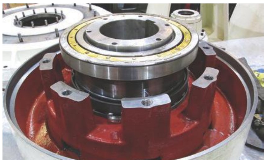
The re-designed thrust bearing arrangement is designed to save around 5 kW of absorbed pumped power as well as increasing the mean time between failure (MTBF).
