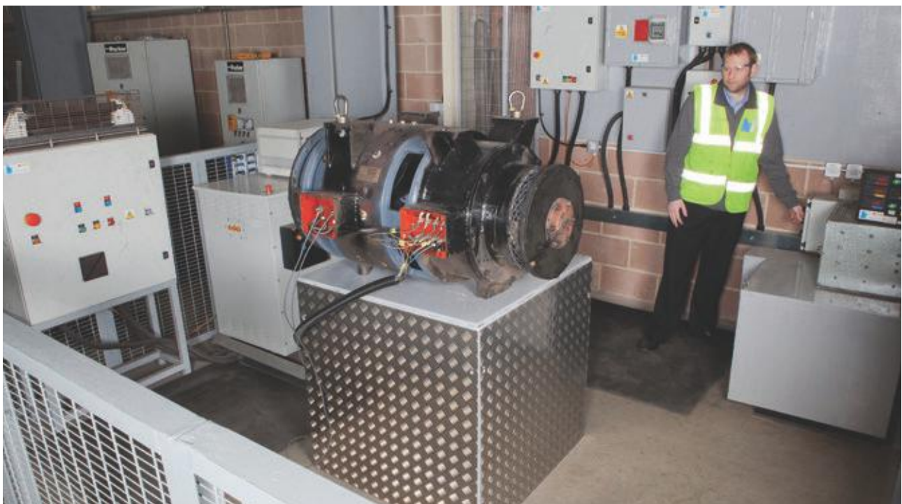
HiTRANS patented full load testing for MA sets
