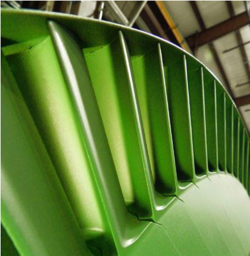
Coatings can be tailored to specific applications and include an aluminium base coat for corrosion protection and a specialist non-stick final layer
