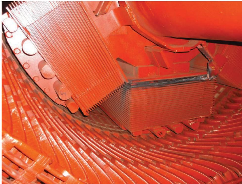
Pole connection damage on the Tata Steel Machine.
