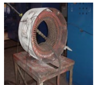
Figure 3. Core testing a stator prior to rewind.
