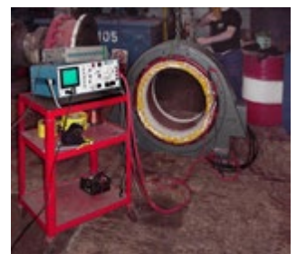
Figure 5. A form coil stator being surge tested.
