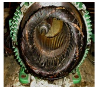
Figure 2. A random-wound stator damaged by contact with the rotor.
