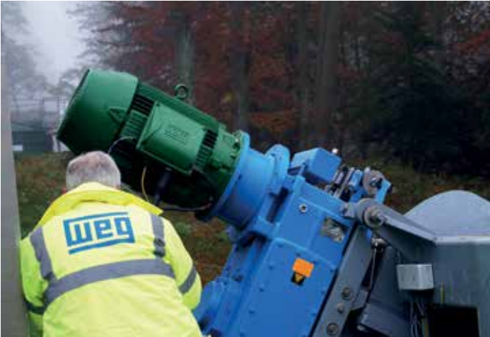
The lighting for the entire house can now be powered using the high efficiency WEG IE3 electric motor driven over-speed as a generator
