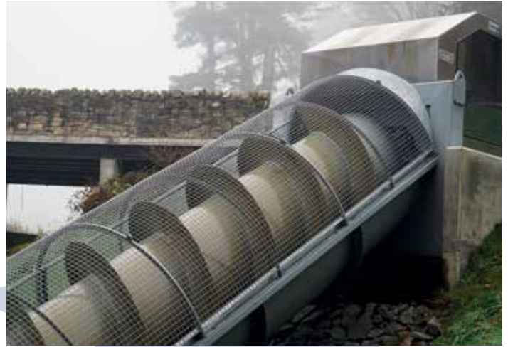
An Archimedes screw, although ancient in principle, is actually a very efficient way of generating power when you have a large volume or flow of water, but low head
