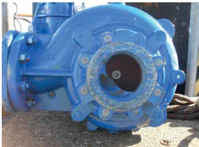
The Hidrostal pumps incorporating the screw centrifugal impeller on site at Corton Church
